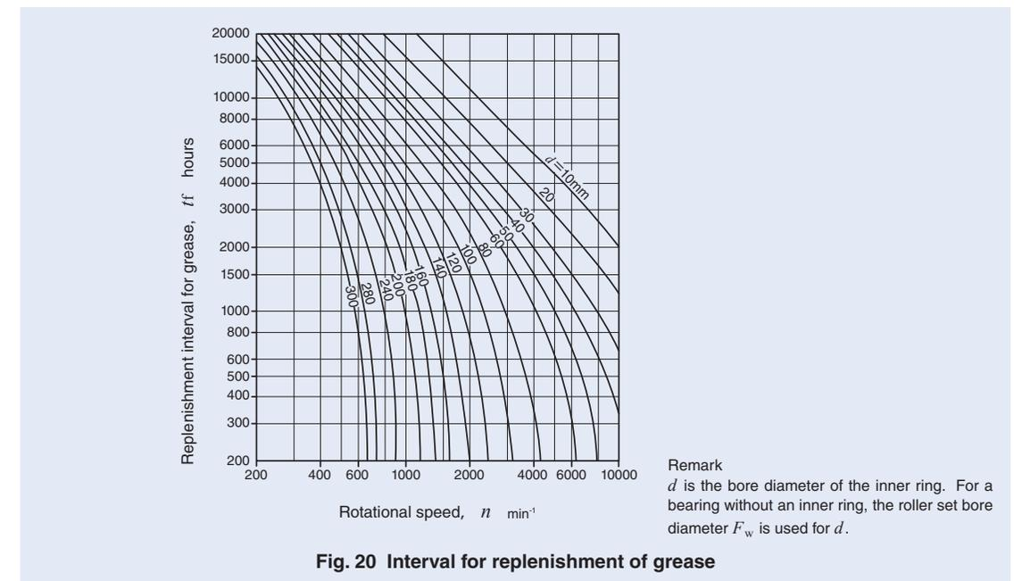
**Fig. 20 Interval for replenishment of grease**
