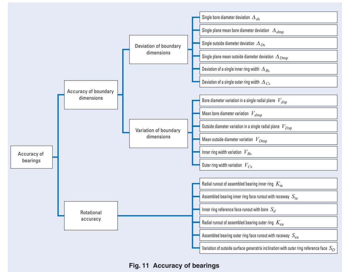
Fig. 11 Accuracy of bearings
