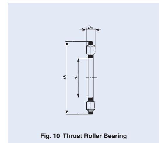
**Fig. 10 Thrust Roller Bearing**
