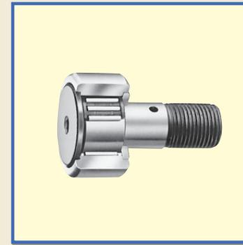
Cam Followers are bearings with a stud incorporating needle rollers in a thick walled outer ring. They are designed for outer ring rotation, and the outer rings run directly on mating cam guide surfaces. Various types of Cam Followers are available. They are widely used as follower bearings for cam mechanisms and for linear motions.
