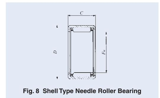
**Fig. 8 Shell Type Needle Roller Bearing**
