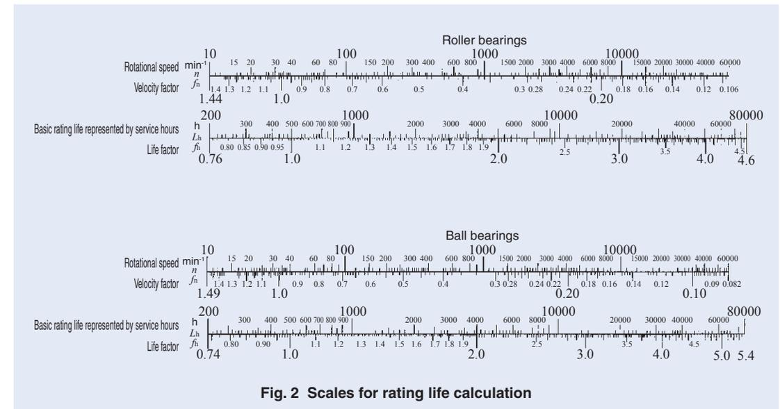
Fig. 2 Scales for rating life calculation
