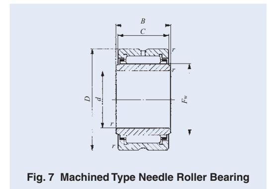
**Fig. 7 Machined Type Needle Roller Bearing**
