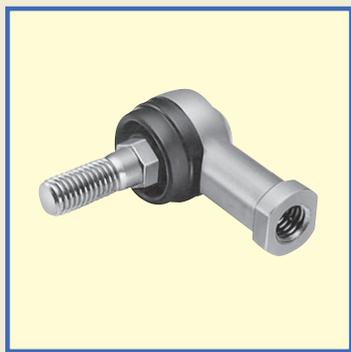
L-Balls are self-aligning rod-ends consisting of a special zinc die-cast alloy body and a studded ball which has its axis at right-angles to the body. They can perform tilting movement and rotation with low torque, and transmit power smoothly due to the uniform clearance between the sliding surfaces. They are used in link mechanisms in automobiles, construction machinery, farm and packaging machines, etc.
