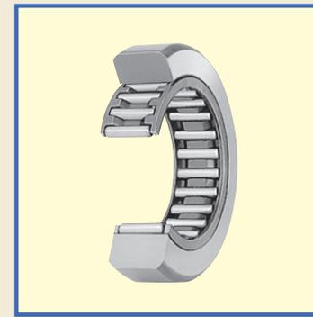
Roller Followers are bearings in which needle rollers are incorporated in a thick walled outer ring. These bearings are designed for outer ring rotation, and the outer rings run directly on mating cam guide surfaces. They are used as follower bearings for cam mechanisms and for linear motions.
